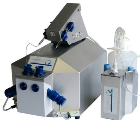
The OROBOROS Oxygraph-2k for high-resolution respirometry, the Titration-Injection microPump (TIP-2k) on top of the O2k, and the Integrated Suction System (ISS) on the right.
