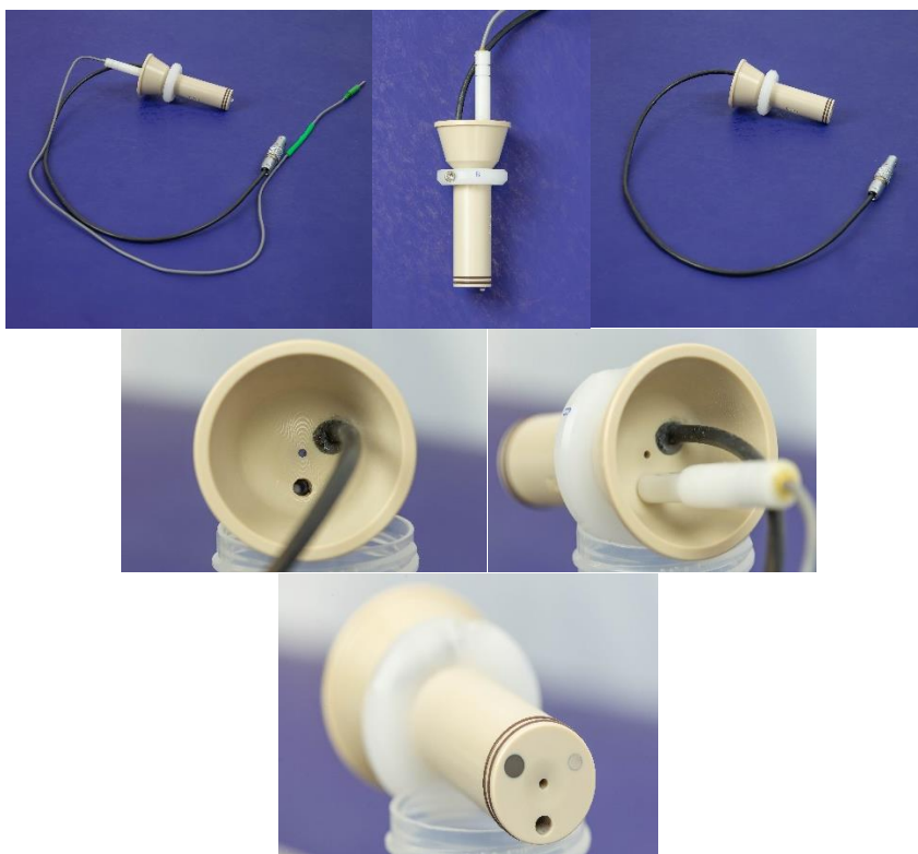
Figure 2. Q-Sensor assembly. First row from left to the right: Q-Sensor with the reference electrode, Q-Stopper without the reference electrode. Second row: Q-Stopper viewed from above without and with the reference electrode. Third row: Q-Stopper viewed from bottom. Glassy carbon electrode (black) and platinum electrode (shiny, silver) are built-in part of the stopper. One gas-escape/titration capillary and an inlet for the reference electrode can be seen.
