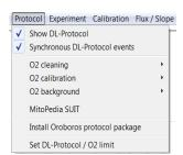
**Top O2k-Applications:** Standardized DL-Protocols are installed with the DatLab software. While the titration steps of these SUIT protocols are fixed, the titration volumes and final concentrations can be adjusted and exported as a customized DL-Protocol by the user (\*.DLPU).
