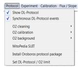
**Top O2k-Applications:** Standardized DL-Protocols are installed with the DatLab software. While the titration steps of these SUIT protocols are fixed, the titration volumes and final concentrations can be adjusted and exported as a customized DL-Protocol by the user.
