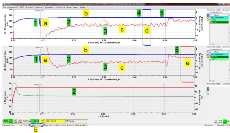
Figure 2. POS Quality control using the DatLab protocol (DL-Protocol) O2 calibration air.DLP : Plot of the 1-hour POS sensor test (above; File 2014-07-24_P4-01_O2-calib.DLD) and oxygen calibration window (below).
