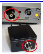
reach the inside of the oxygraph. BNC type connectors are used frequently for attaching potentiometric electrodes (pH) and therefore also used for the pX channel in the MultiSensor extension. By the nature of the BNC plug it is possible for the operator to touch the outside channel and thereby cause an ESD.
