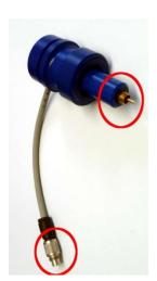
Within the stainless steel O2k housing, internal electronic components are well protected from ESD. However, during chamber assembly, membrane change, or trouble shouting, the polarographic oxygen sensor (POS) has to be disconnected from the POS connector and the POS connector is disconnected from the main unit. This means that one or both electric connections of the POS connector are exposed to the environment and ESD damage is possible.
