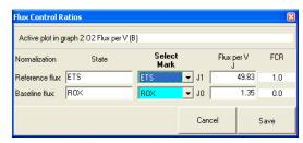
Flux control ratios (FCR) can be plotted after defining the (maximum) reference flux,  $J_1$  (e.g. ETS capacity, noncoupled), and a (minimum) baseline flux,  $J_0$  (e.g. flux after inhibition by rotenone and myxothiazole, ROX) in the window Plots \ Flux control ratios. After selecting the
